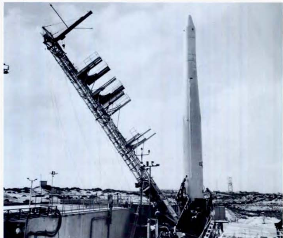
A Thor missile, with gantry to the left, used in an ICBM weapon system simulation test on Johnston Atoll, August 1970. Some Los Alamos personnel served in an advisory role to the Task Force commander, while others aboard the Los Alamos flying-diagnostic-laboratory aircraft observed the missile launching and flight. This readiness exercise served as a very valuable and effective checkout of the missile system.
